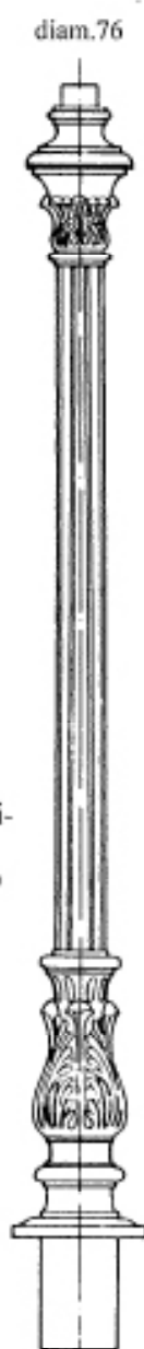
THK-640 candelabra-top Fixed with Stainless-steel set screws Material: gray cast iron weight: 80kg. (176 lbs.)
